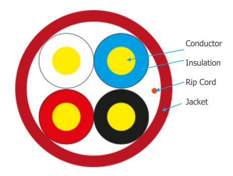
Inner Conductor: 0.77±0.005mm, Solid Bare Copper, OFC
